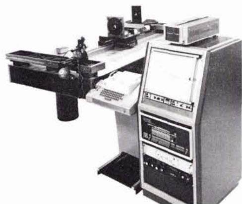
FIG. 3. The equipment must have a fairly high degree of automation. A small mini-computer will almost certainly be part of any modern working lens-test equipment.
