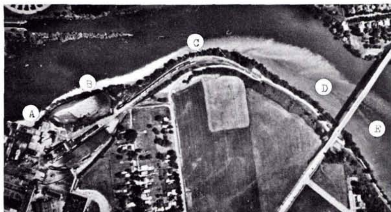
FIG. 1. Photograph of a waste discharging from a paper mill. Samples were taken at A, B, C, D, E, and at many other places in the plume. Results from analyzing these samples are shown in Figure 6.
