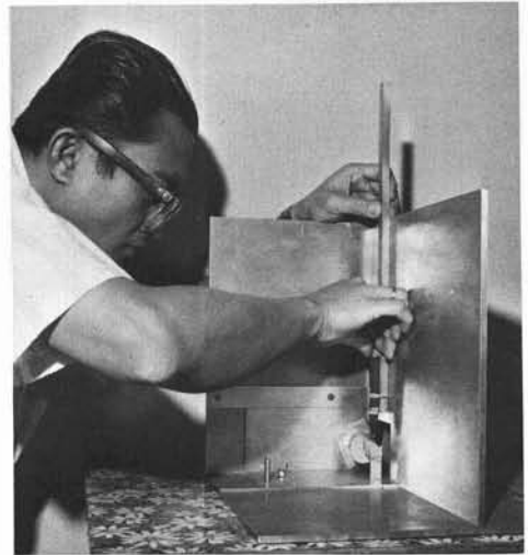
FIG. 6. Placing dots on the mold's surface using a home-made device.
