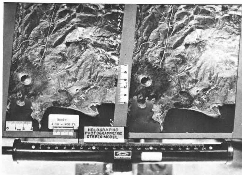
FIG. 18. A stereopair containing an explosively produced crater.
