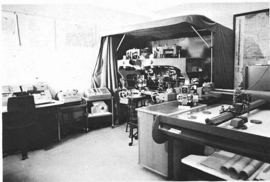
FIG. 6. Wild A7 modified for hologrammetric mensuration and mapping.
