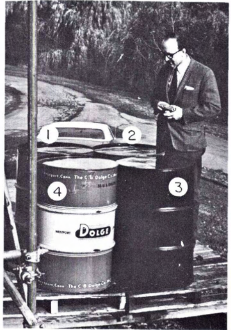
FIG. 3. Barrel configuration at foot of scaffold: (1) water, (2) Diesel fuel, (3) gasoline, and (4) spent lubricating oil.
