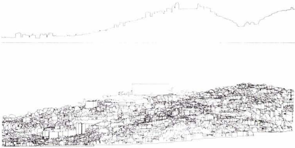
FIG. 5. Thiers. East-west section obtained by photogrammetric plotting.
