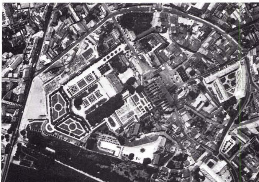
FIG. 1 and 2. A portion of an aerial photograph, located 9 cm from the centers of the photograph from which it was taken. Taken with a lens of 152 mm focal length. Limoges, city area near cathedral. (South at the top).
