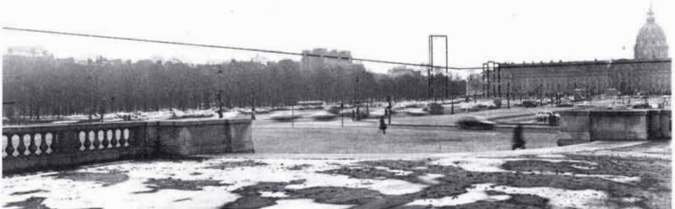
FIG. 15. Protection of the area of the Invalides in Paris. Perspective drawing, by inverse photogrammetry, of outlines of a proposed building project.
