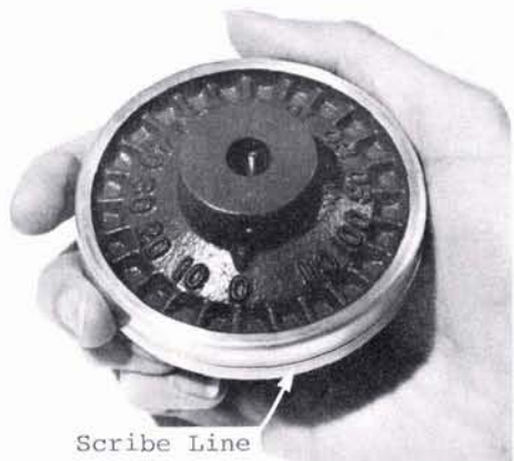
FIG. 2. Graduated handwheels have been added to the elevating screws.
