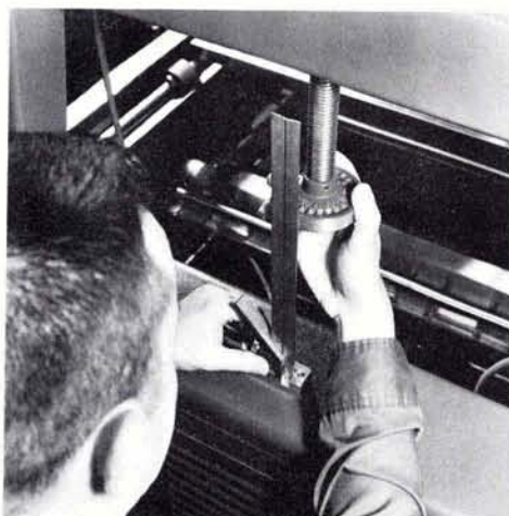
FIG. 3. With the graduated handwheel and a square, the elevating screw becomes a micrometer.
