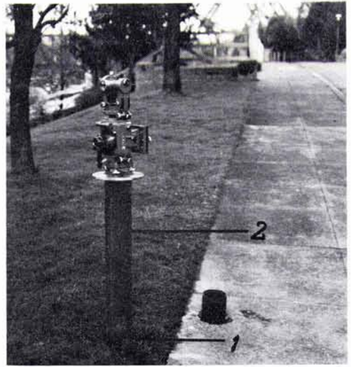
FIG. 4. A pipe stand arrangement can be used for repeatedly setting a phototheodolite over the same ground point.
