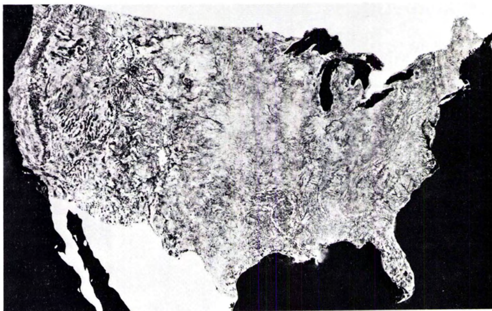
FRONTISPIECE. First satellite mosaic of the conterminous U.S. consisting of 595 cloud-free ERTS-1 satellite images compiled for NASA/GSFC by USDA Soil Conservation Service. Original is 10 x 16 feet at a scale of 1:1,000,000.
