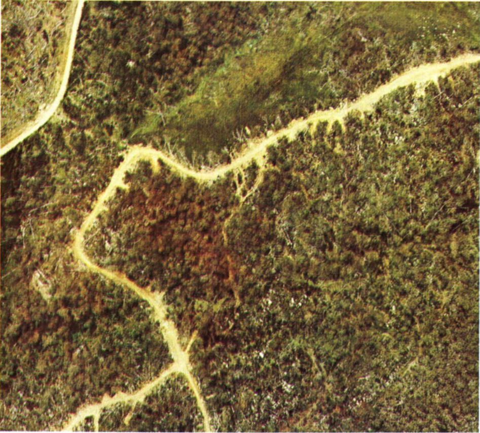
PLATE 1. A print enlarged 2\times from a 70-mm negative exposed over the study area. The photograph is from the best combination of film, illumination and scale: color, under cloud, 1:4000. The rock outcrops show up quite clearly on this combination in one of the areas of lowest crown density (approximately 25 percent).
