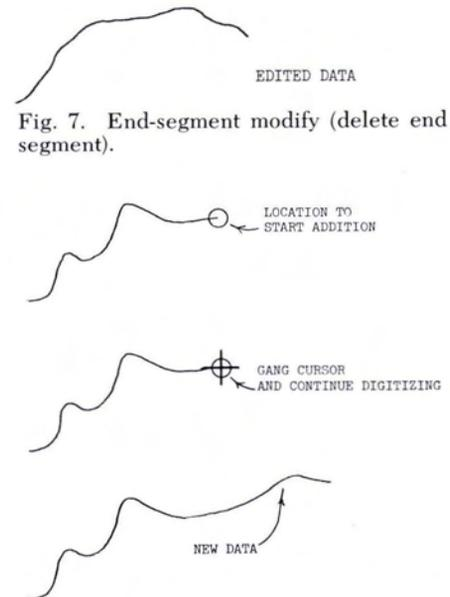
FIG. 8. End-segment modify (extend end segment).
