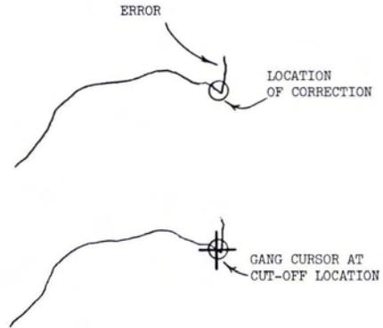
Fig. 7. End-segment modify (delete end segment).
