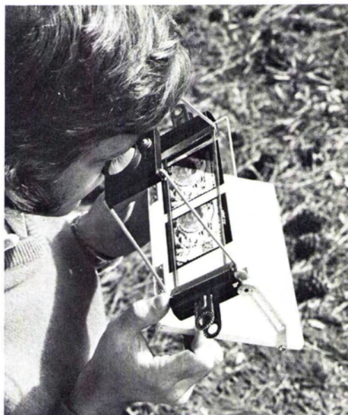
FRONTISPIECE. The field transparency viewer in use with a stereo pair of 70mm aerial photos.
