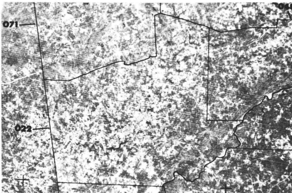
FIG. 2. A 1:1,000,000-scale transparent overlay was used to outline Carroll County, Georgia, on Earth Resources Technology Satellite bulk color composites; this portion of ERTS scene 1264-15445 is enlarged to a 1:500,000 scale.
