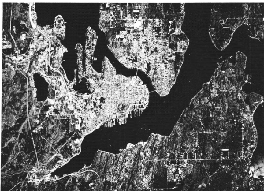
FRONTISPIECE. Unmagnified high-altitude image of Bremerton, Washington (scale 1:135,000). Original image recorded on false-color-infrared reversal film.
