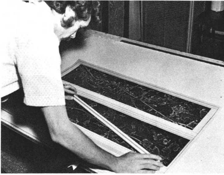
FIG. 3. Checking scale on plan-and-profile sheet on utilities map.
