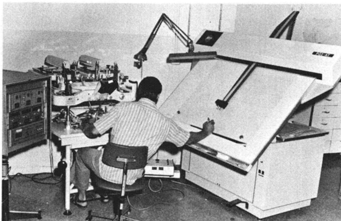
FIG. 4. Kern PG-2 stereoplotter, teletype terminal, digitizing unit consisting of Datas 303 Data Transfer System, DGC 400 Scaling Translator and a digital readout, all at one station.
