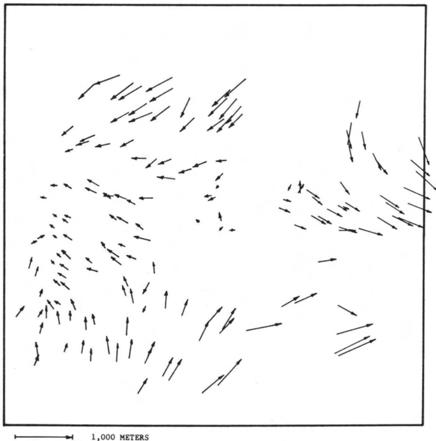
FIG. 3. Distortion map from conformal transformation to State Plane coordinates frame E-1202-16381-4.
