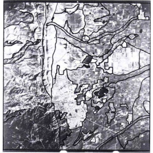
Fig. 2. Black and white infra-red aerial photograph of the City of Boulder. Photomorphic areas are delineated in black.
