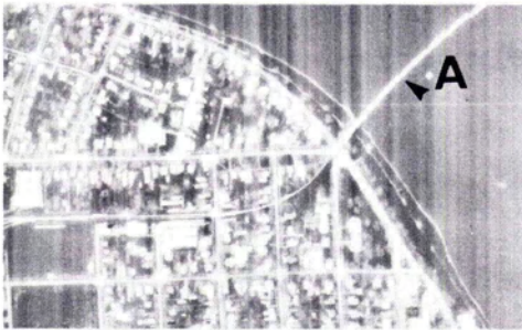
FIG. 3. Sample infrared imagery rectified. Notice the elimination of the distortion in detail A.
