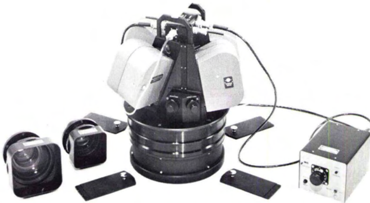
FIG. 6. Multiband camera interconnected for operation. Intervalometer in the right foreground, four film magazines in place and loaded with film, 4-inch focal length lens on extreme left, and 6-inch focal length lens next to the camera base. Ring mount of the camera will fit standard aerial camera hatches.
