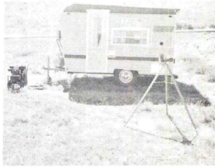
FIG. 3. Field spectrometer trailer and support equipment. A tripod-mounted, first surface mirror (a and b) was used to fold the horizontal field-of-view of the spectroradiometer down onto the sample. A 3500-watt power plant supplies field power. A cable locker (not shown) has been added atop the rear bumper to store the trailer's main power cable (90 m), a remote site power cable (90 m), and a remote site data and communication cable.
