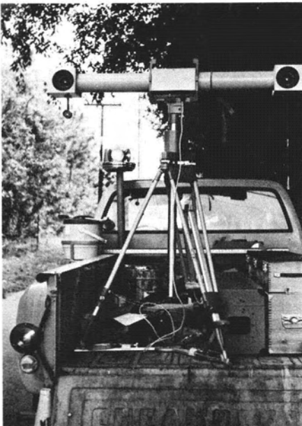
FIG. 1. Stereometric camera mounted on a pickup truck.
