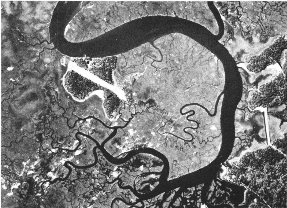
FIG. 7. Portion of an orthophoto used in the preparation of an orthophotoquad. (Northward is toward the bottom).
