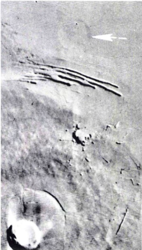
FIG. 10a. Mariner 9 picture (DAS 07111198), shows false detail created during computer image processing (arrow).
