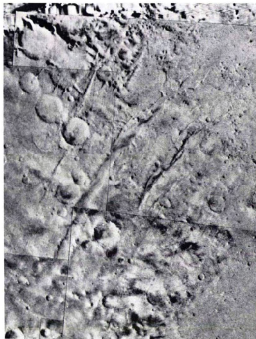
FIG. 13. Part of a typical mosaic used for horizontal control during the drawing process (MC-13 Syrtis Major).
