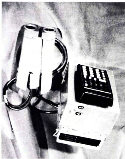
FIG. 2. The prototype hand-held biomass meter, consisting of a radiometer with two probes interfaced to a pocket calculator through a programmable data collection digital interface.
