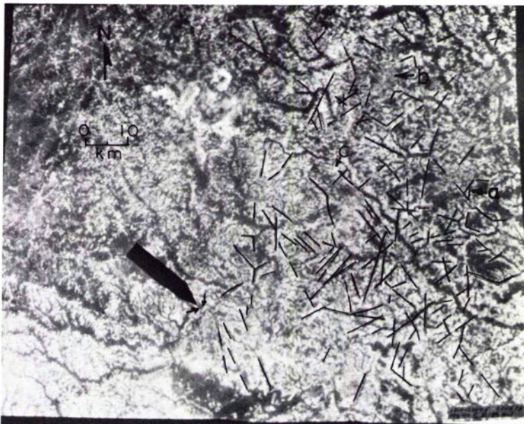
FIG. 5. Lineaments, North Carolina coastal plain. (a) Fountain Quarry; (b) Rocky Mount with several quarries nearby; (c) Wilson. Large arrow points to general location of Coats Scarp, and smaller arrows show its approximate extent. LANDSAT-1 Image 1314-15204-5, 2 June 1973. Picture made using 1:1,000,000-scale transparency, transmitted daylight and Ektachrome ASA 64 film.
