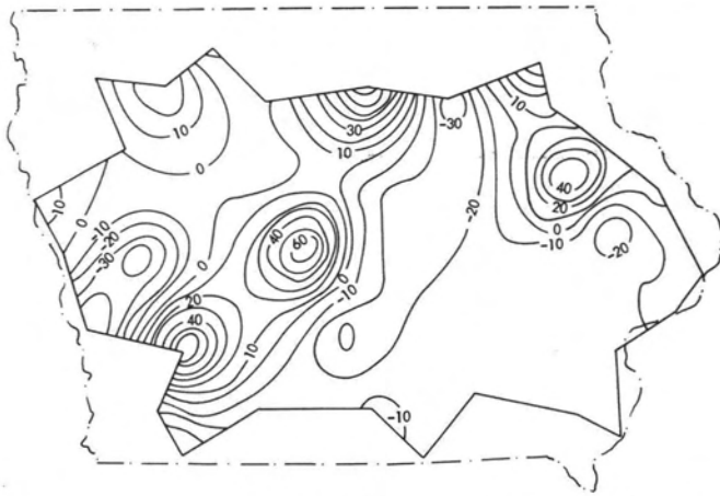
FIG. 11. Free air anomaly map of Iowa using the reciprocal distance as a kernel in a multiquadric harmonic function (depth of 43 point masses, 30 km).
