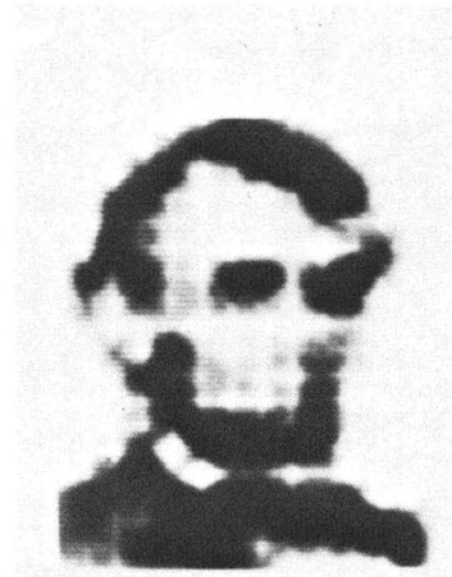
FIG. 16. Photograph of off-line TV reconstruction of the Lincoln image with a one-time 4 \times 4 coefficient matrix inversion.
