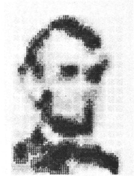
FIG. 14. A multiquadric reconstruction of the Lincoln image with a one-time 4 \times 4 coefficient matrix inversion.
