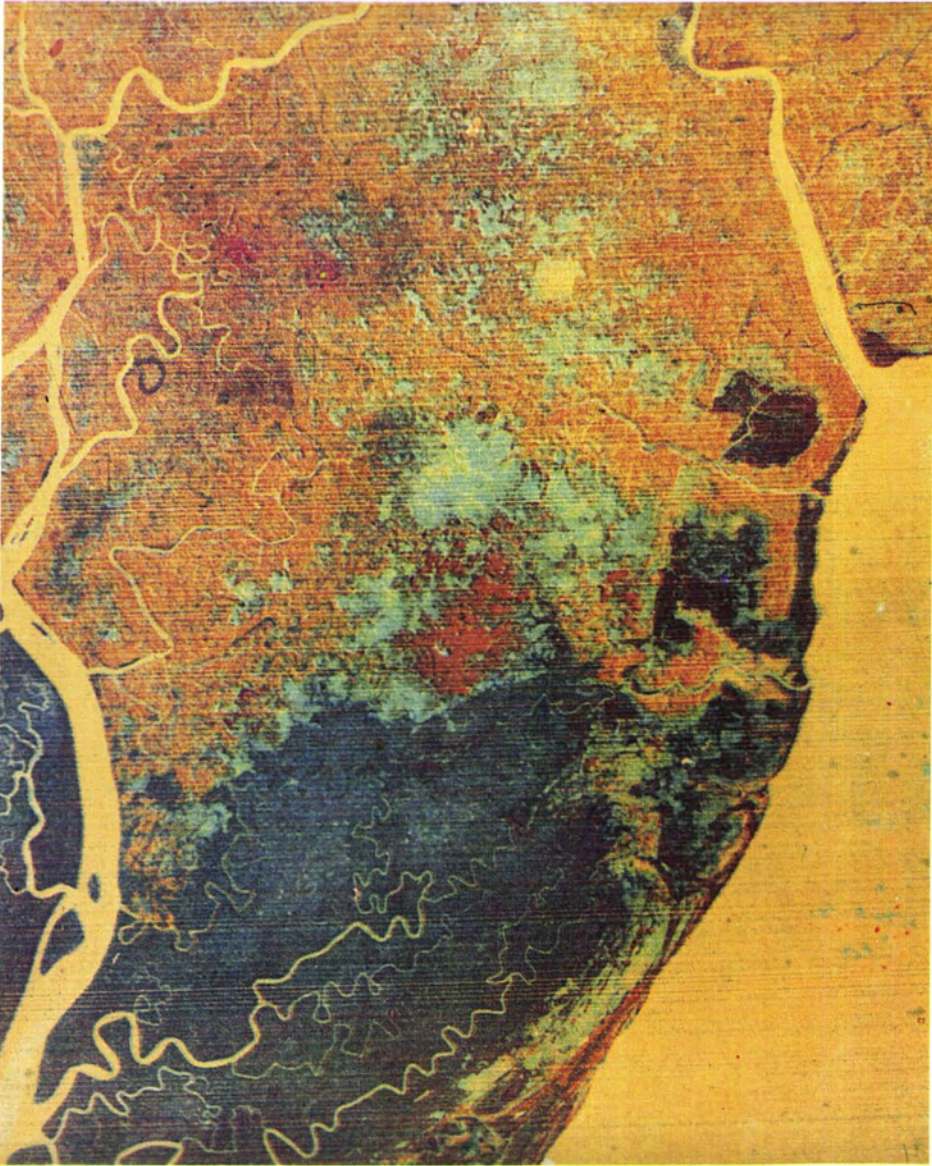
PLATE 1. This illustrates the type of color composite which can be generated by the CIE Color Prediction Model. The scene incorporates part of the Irrawaddy River delta in Burma southwest of Rangoon. The image scale is approximately 1:400,000 (scale of Transparency was 1:250,000). (LANDSAT-1 bands 4+ cyan, 5- yellow, 7- magenta; NASA Accession Number E-1513-03262.)
