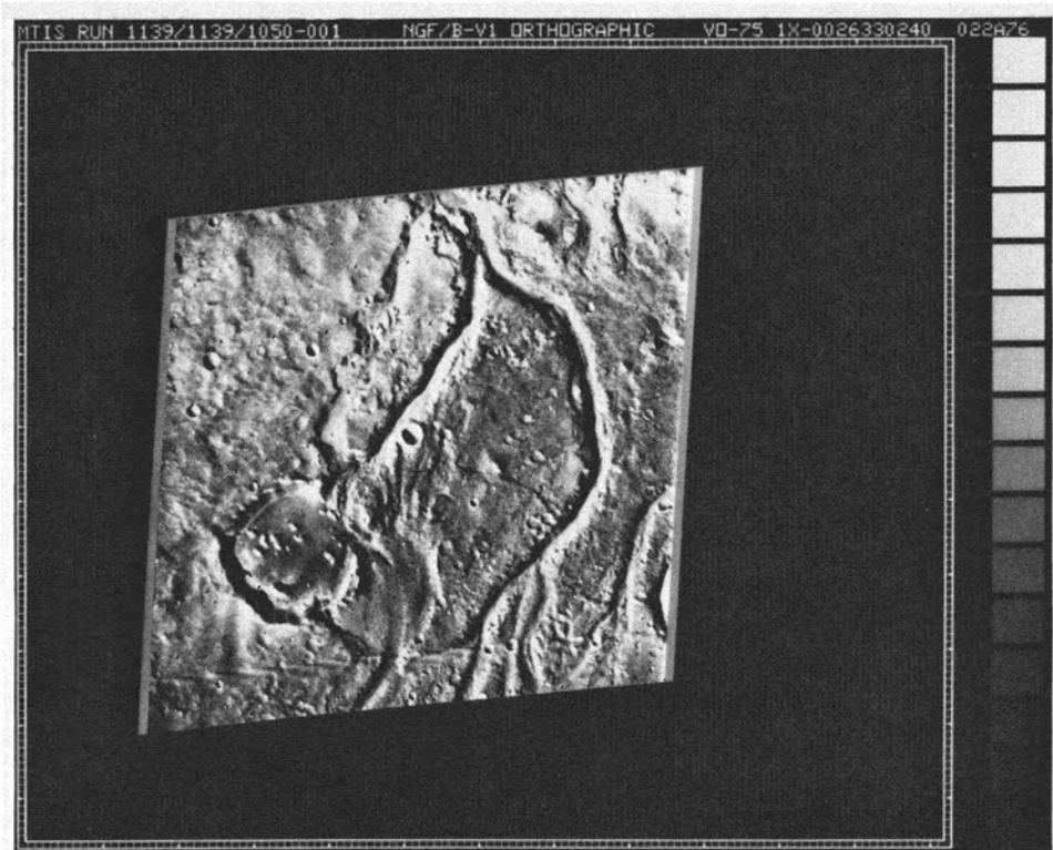
FIG. 1. Typical Viking Orbiter rectified picture (orthographic), showing image area, pixel scales (10 pixels per division), and picture identification numbers at top right.
