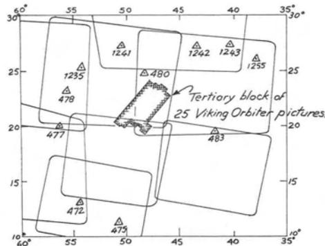
FIG. 2. The Mariner 9 secondary block showing Davies' primary points and incidence of tertiary block.
