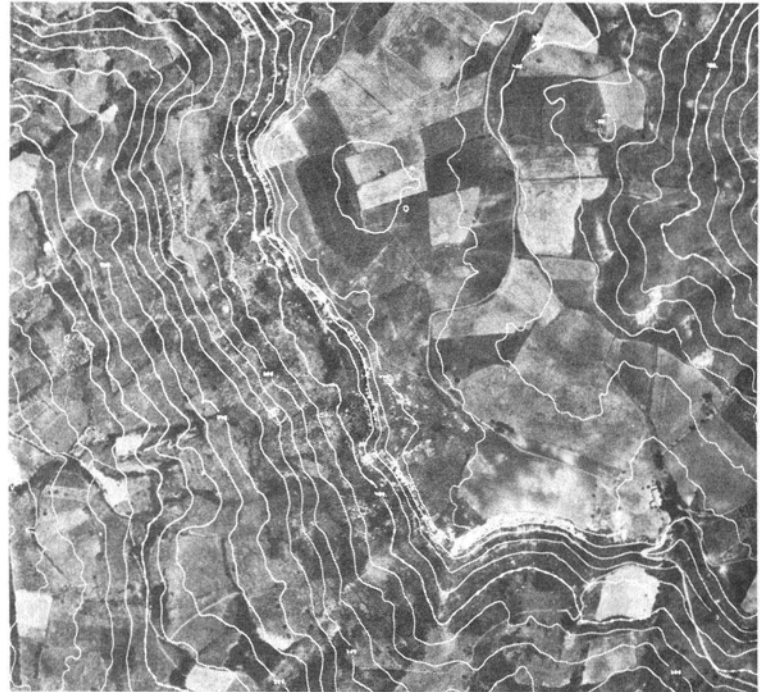
FIG. 4. GPM II orthophoto with plotted contours. This orthophoto is a 2.3-times enlargement of a portion of a GPM orthonegative (reproduced herein at 0.75\times ). Differential rectification is based on a matrix of points with the same spatial frequency as the numbers in the DTM in Figure 1.
