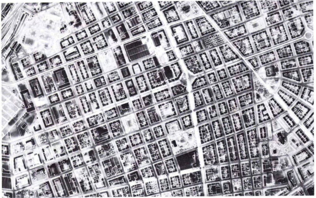
FIG. 4. Extract from rectified MSS image with map details from the Vienna City Maps superimposed, scale 1:10 000.
