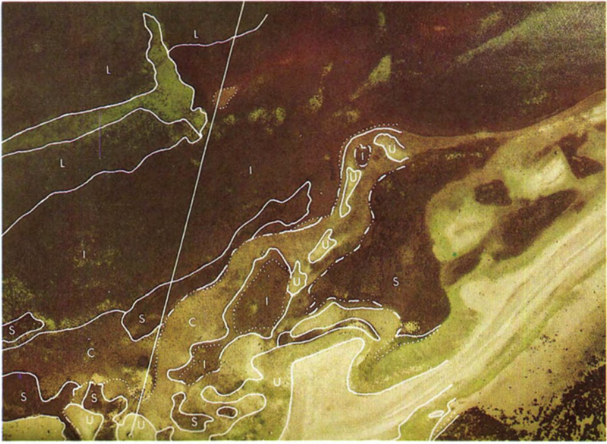
PLATE 1. Portion of natural color (2445) print of intertidal and subtidal vegetation at low tide (Kye Bay, Vancouver Island) at scale of 1:5,000. Overlay indicates survey transect location and seaweed vegetation units defined from ground data. Legend: C = Cryptosiphonii woodii I = Iridaea cordata L = Laminaria groenlandica S = Sargassum muticum U = Ulva spp. Dashed line = water line (+0.6 m).
