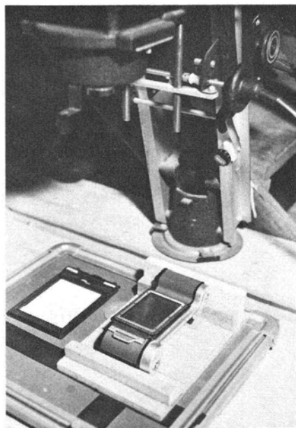
FIG. 1. Film holders for macrophotography under the enlarger: left, 4 by 5 sheet film holder; right, 120 roll film holder.
