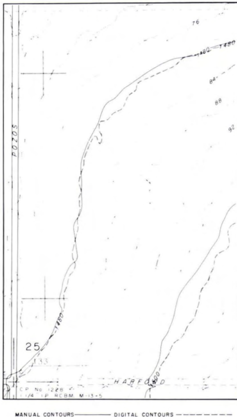
FIG. 1. Typical difference between manual contours and digital terrain contours.
