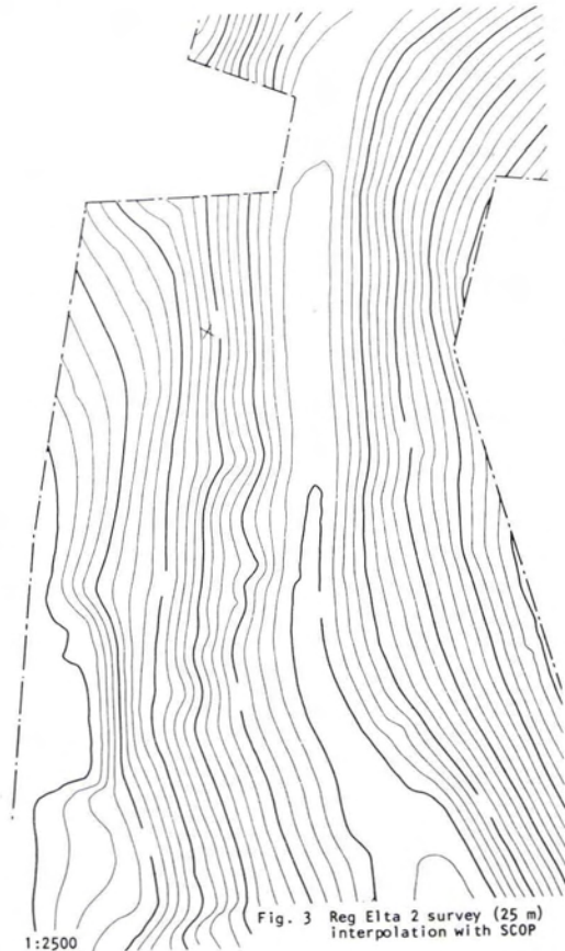
FIG. 3. Reg Elta 2 survey (25 m), interpolation with scop.
