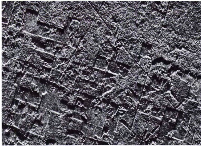
FIG. 4. Enlargement ( 6\times acquisition scale) to a scale of 1:67,000 of a portion of a SLAR image. Depression angle is approximately 9^\circ . Note shadows east by forest across adjacent pasture land.
