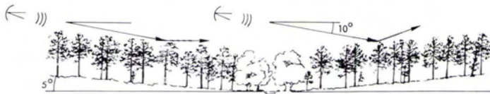
FIG. 5. Schematic presentation showing imaging at mid-range depression angle across a typical valley in the North Louisiana Salt Dome area.
