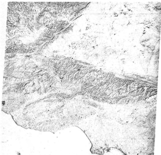
FIG. 4. Enhanced image of the greater Los Angeles area. Linear features associated with systems of highways and with agriculture generally stand out as lines of dark spots, and lineaments of geologic interest as light lines or as linear zones separating areas of different texture.
