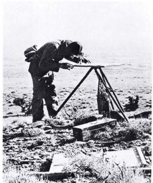
FIG. 3. Topographer illustrating the use of a planetable, ca. 1905.
