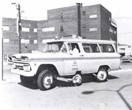
FIG. 4. The elevation meter, developed in the early 1950's, afforded an automatic means of obtaining elevations of points along roads.
