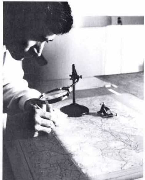
FIG. 10. Final preparation of a contour-line scribe sheet used in the production of a usgs topographic map.
