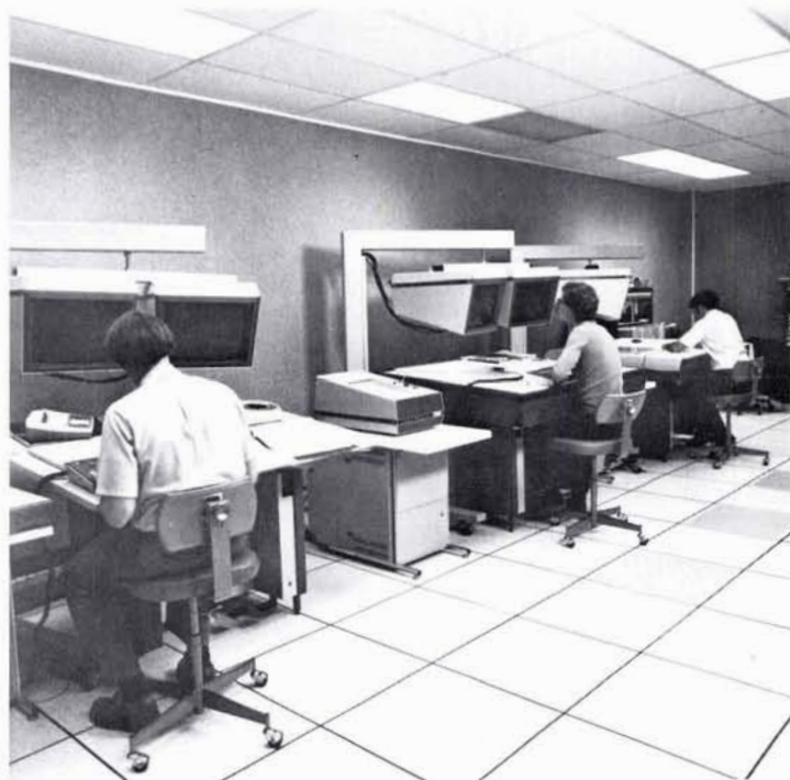
FIG. 12. Digital map data collected with two- and three-axis systems can be interactively edited and revised on the Digital Data Editing System.
