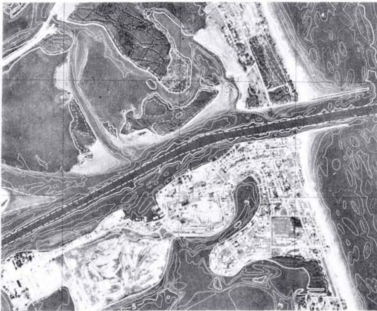
FIG. 1. This portion of the Fort Pierce, Florida 7½-minute orthophotoquad shows nos bathymetric data added to usgs orthophotography.
