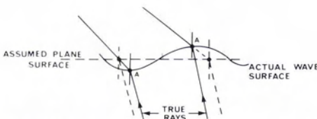
FIG. 7. Effect of assuming a plane air/water interface on the position of the surface point A; component due to variation in water depth.
