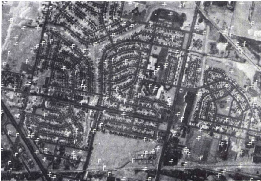
FIG. 3. Black-and-white print of one band of the original Noyes Creek image illustrating the marking procedure used in verifying the accuracy of the computer classification.
