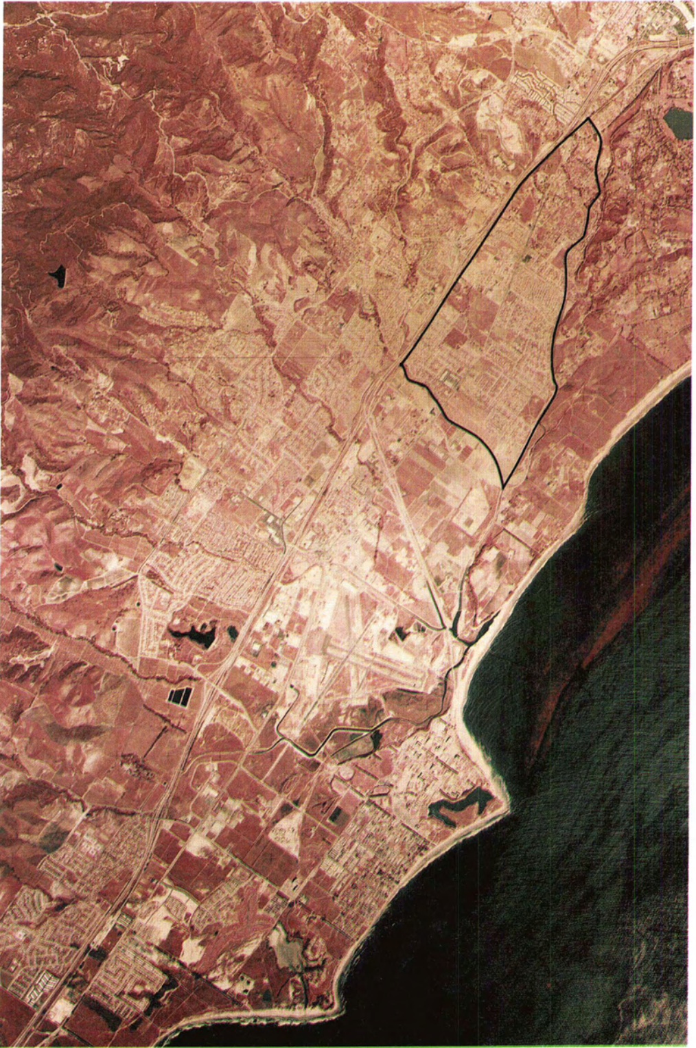
PLATE 1. The location of the study area, census tract 30.03 in the Santa Barbara, California, Standard Metropolitan Statistical Area, has been outlined on the NASA high altitude color infrared aerial photograph taken in April 1971 at a contact scale of 1:63,360. This photo is illustrative of the type of imagery from which our estimates of numbers of residential units were made.
