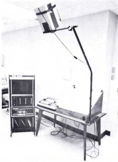
FIG. 4. The SHM (now ATC) Rad-8 computer system. An opaque projector (upper center) has been mounted to project Polaroid photographs onto the graphics terminal (right).
