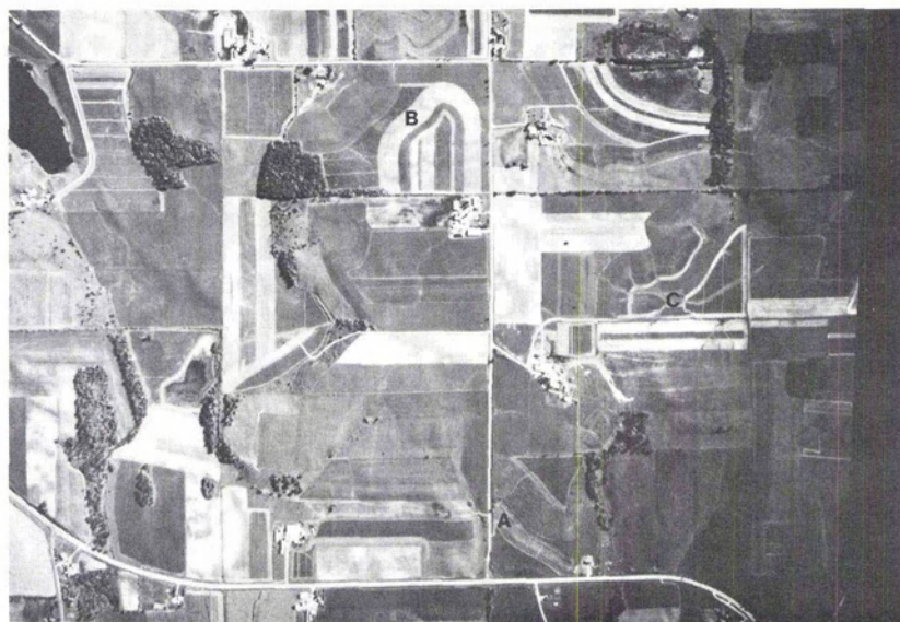
FIG. 1. Black-and-white copy of a color infrared photo showing the predominant erosion control practices in Pheasant Branch Creek watershed. A = contour tillage, B = contour strip cropping, and C = grass waterways. (Scale = 1:24,370)
