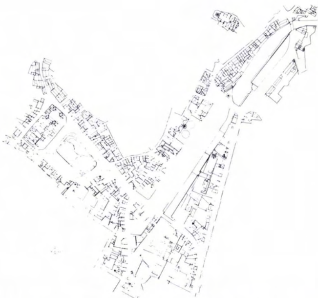
FIG. 5. Aurillac, town center, plan survey. (N.B. Figures 5-8. The original plots at a scale of 1:1000, obtained by digital plotting of 1:8000 scale aerial photographs, computation with the TRAPU program, and automatic drawing, were carried out by the I.G.N. for Mr. Jean-Pierre Duthoit, architect.)
