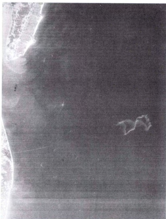
FIG. 2. Acid waste plume visible in Landsat mss band 4 imagery on 24 February 1976 (3 hours and 23 minutes after dump completion).
