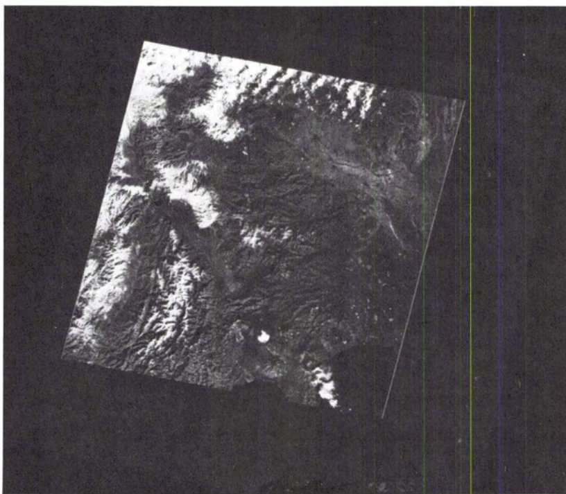
FIG. 7. Geometrically corrected result of "Toukai" (Landsat-1, 15 December 1972) projected to the conformal conic projection.
