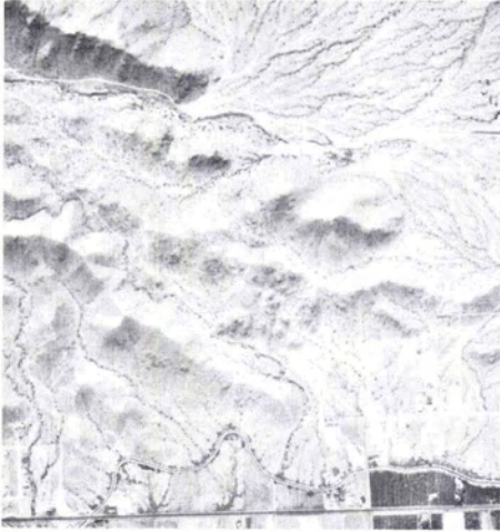
FIG. 1. Aerial photograph of the site of the digital terrain model. The stereo imagery from which the digital terrain model was produced was taken over Phoenix South Mountain Park, just outside Tempe, Arizona. This image, which is 2048 by 2048 picture elements in size, represents a two-inch square section digitized from the original photo by the U.S. Army Engineer Topographic Laboratories.
