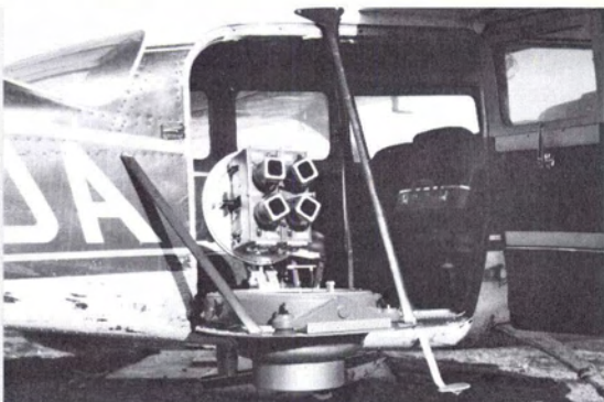
FIG. 2. Hasselblad camera system in its 'up' position. The bubble has been removed and the forward door opened for this photograph. Narrow band multispectral interference filters are fitted to the four lenses.
