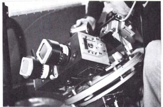
FIG. 3. Changing a magazine on one of the Hasselblad cameras. With the hinged mount adaptor, and cameras housed in two banks, this is easily accomplished while flying. The alignment screws for the camera in the foreground are seen on the end of the hinged camera support.
