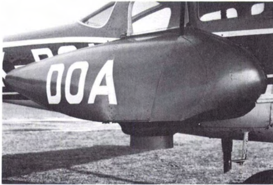
FIG. 1. Streamlined aluminium bubble attached to the side of Cessna 206. The driftsight can be seen protruding through the floor of the aircraft.
