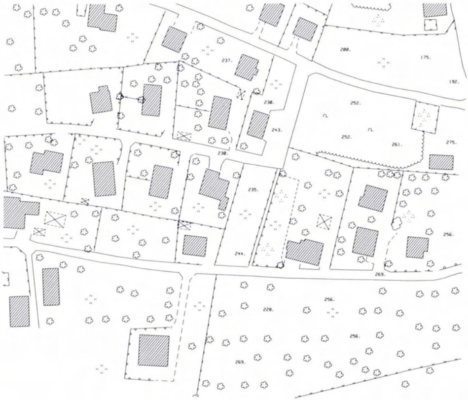
FIG. 8. Direct plot of a 1:1000 site plan. The line types and symbols are those required by a private firm in Germany, derived at short notice by the operator. The shading and the spot heights were plotted automatically. Mapping was completed in about a third of the time that would have been normally required (compared with a plot produced without computer system or digital plotting table).
